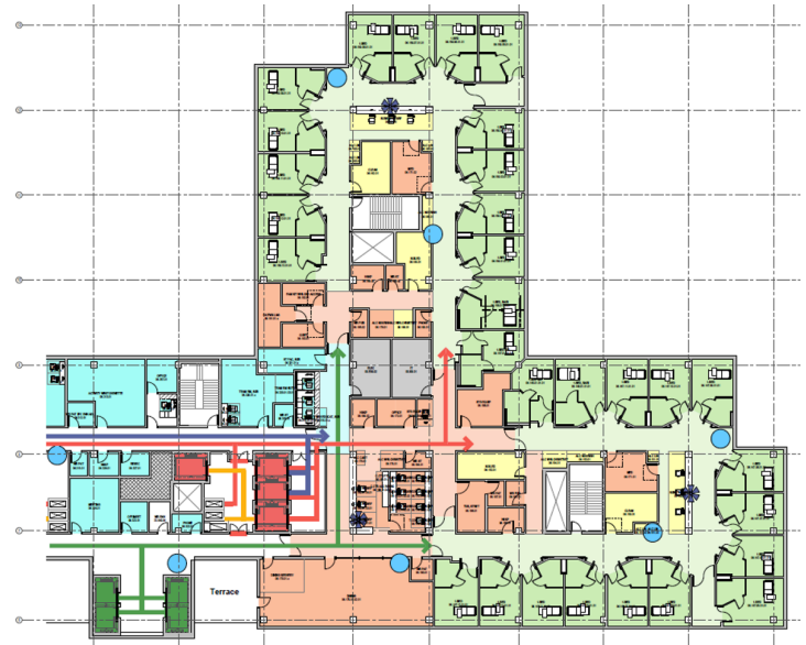
Sample Illustrative Schematic Design, courtesy of Stantec. This is an example of the type of detail that can be looked at inside one department, including doors, beds and equipment inside the rooms.
