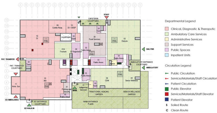
Sample Block Diagram plan, courtesy of Stantec. This drawing shows all programs and services on an entire floor and their locations in relation to other programs and services as well as entrance points, elevators and the hallway circulation route.
